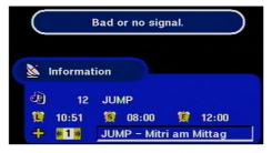
"Bad or no signal" indicates that there is a fault in the reception system or in the receiver settings or the transponder is not transmitting. Instead of the **I** the channel identifier shows a satellite antenna together with the message "bad or no signal". Check the SAT-IF connection and the LNB configuration. As an aid, refer to
